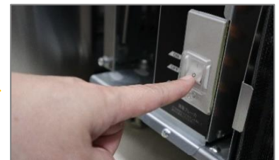
④ After descending, turn off the earth leakage breaker, disconnect the power plug, open the door, and dry the inside of the refrigerator.
